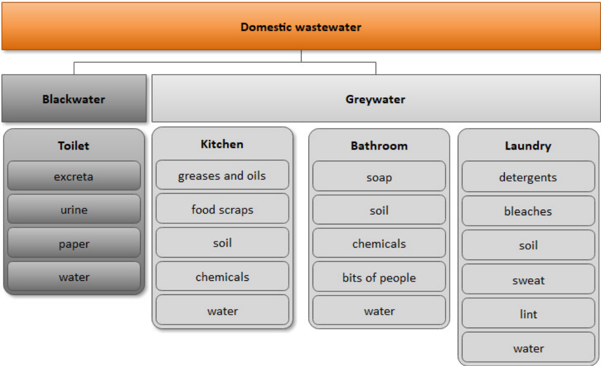
Figure 3. Origin of domestic wastewater and its content.
